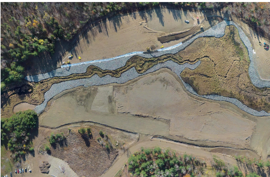
Area A during remediation. The creek and marshland running through the site were protected due to natural filtration and buffering qualities. GCL was brought as close to the shoreline as possible where riprap was installed to prevent any further erosion of this ecologically sensitive area.
