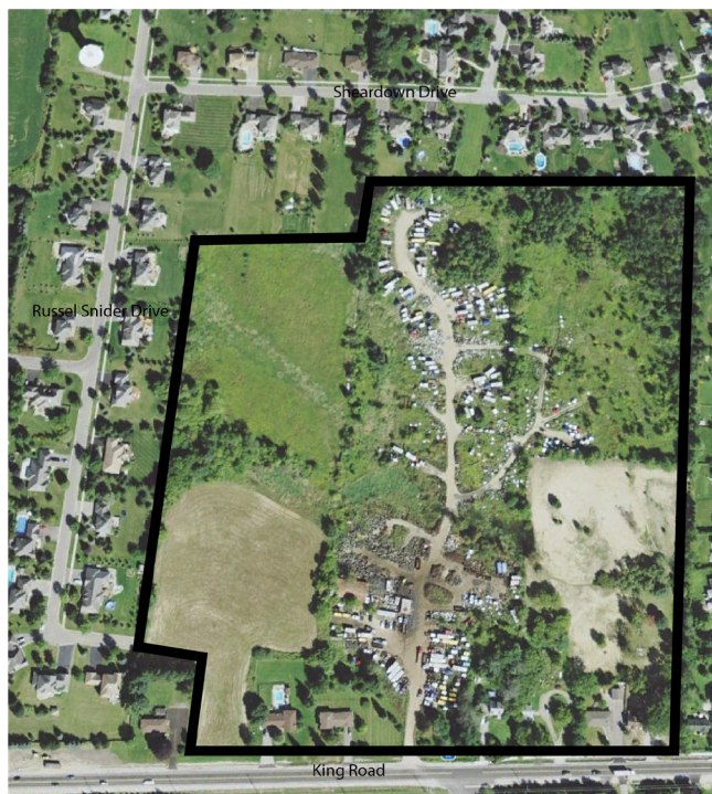
Figure 2. 2009 Historical Satellite view of the future development boundaries. Various AST, Fill piles and automobiles can be witnessed in the central section of the property.
